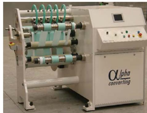
**ALPHALAB TWIN – a narrow width slitter with individual dust extraction for each knife.**
