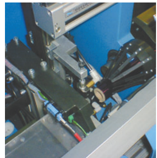
Fully automated core labelling, roll sleeving and heat sealing direct from the machine.
