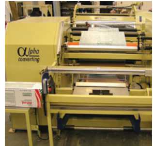
In-line application features end of line winding and boxing for continuous operation.
